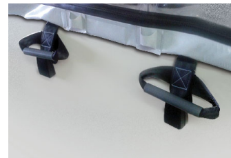
Lifting handles in the base of the chamber
